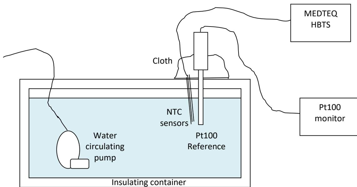
The Pt100 probe and NTC thermistors should be immersed to a depth of at least 7-8cm, with the opening covered to minimize the ambient influence. Alternately they may be completely immersed for best accuracy.
