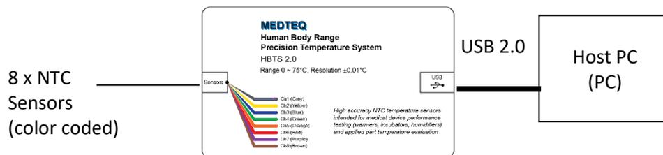
USB module measures sensor data and streams to the PC for further processing and display.
